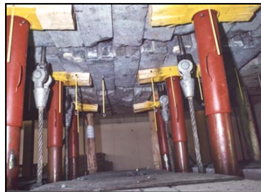
Figure 3: During the energy impulse no blocks were dislodged into the stope area.
